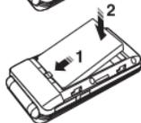
3. To remove the battery, lift the bottom of the battery up (1) and remove (2) the battery. Push the SIM card in the direction of the arrow as shown.
