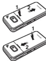
2. Insert the SIM card into the slot. The gold contacts of the SIM card should go against the metal contacts of the phone. Put the contacts of the battery into the hole located at the upside of the unit insert (1) and press the bottom side of the battery (2) until you hear the "click".
