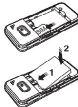
3. To remove the battery push the bottom of the battery to upwards (1) and remove (2) the battery. Pull the SIM card in the arrow direction as shown.
