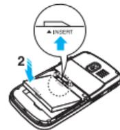
Put the contacts of the battery into the hole located at the bottom of the unit insert and press the upper side of the battery until you hear the "click". Make sure you align the gold contacts at the battery end with contacts on the phone. If the contacts at the battery are not properly aligned, damage could occur to the phone and the battery.
