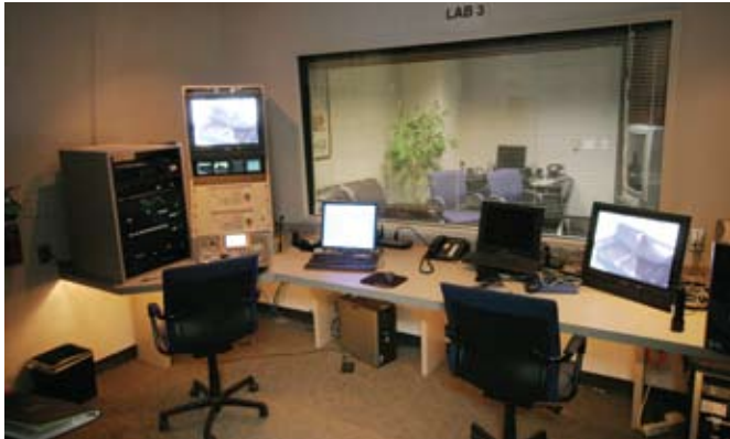
Human Factors Lab: A control room where experimenters observe customers interacting with AT&T products and services.
