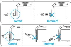
2. To remove the adapter connection, pull the adapter away.
